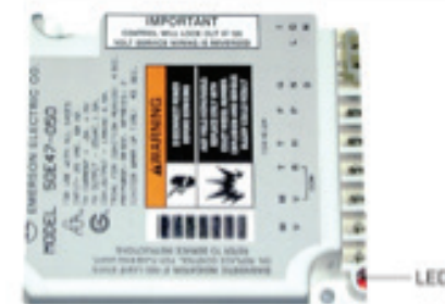
LED ON = FAILED CONTROLLER LED FLASHING = EXTERNAL COMPONENT FAILURE CONTROLLER WITH MINIMAL DIAGNOSTICS
